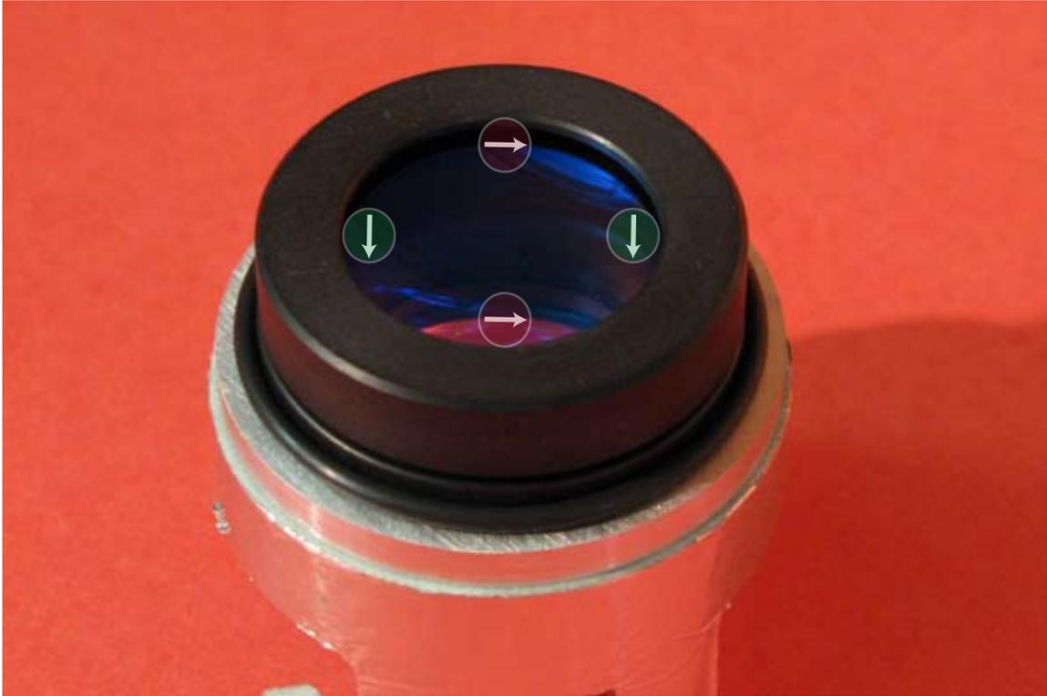
Figure 7.5: The four beams that create the 2D square lattice are shown entering the microscope objective. The polarization of the beams is indicated by the white arrows and chosen such that the interference pattern produced at the focus of the objective is linear at the position of the atoms.
